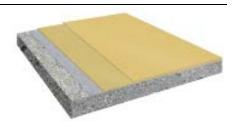
1x Sikalastic $^{\circ}$ -560 MY + 10% water = 0.4 kg/m $^{2}$  2x Sikalastic $^{\circ}$ -560 MY = 0.50 kg/m $^{2}$ /layer Build up:
